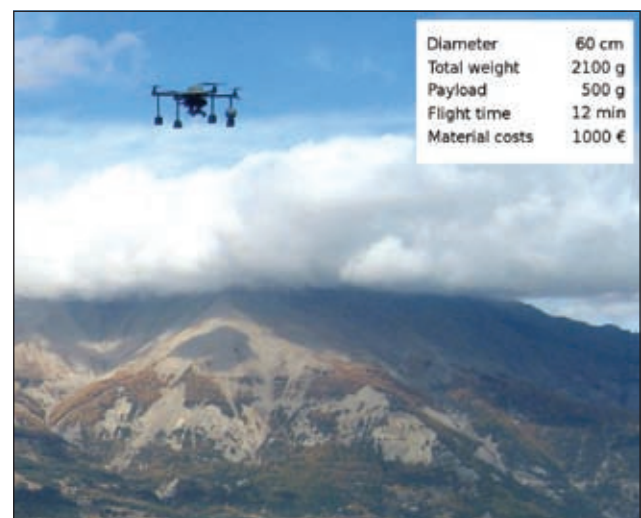
Figure 5 Quad-rotor system for remote sensing and its main characteristics. Here in use at the mudslide in Super-Sauze.
